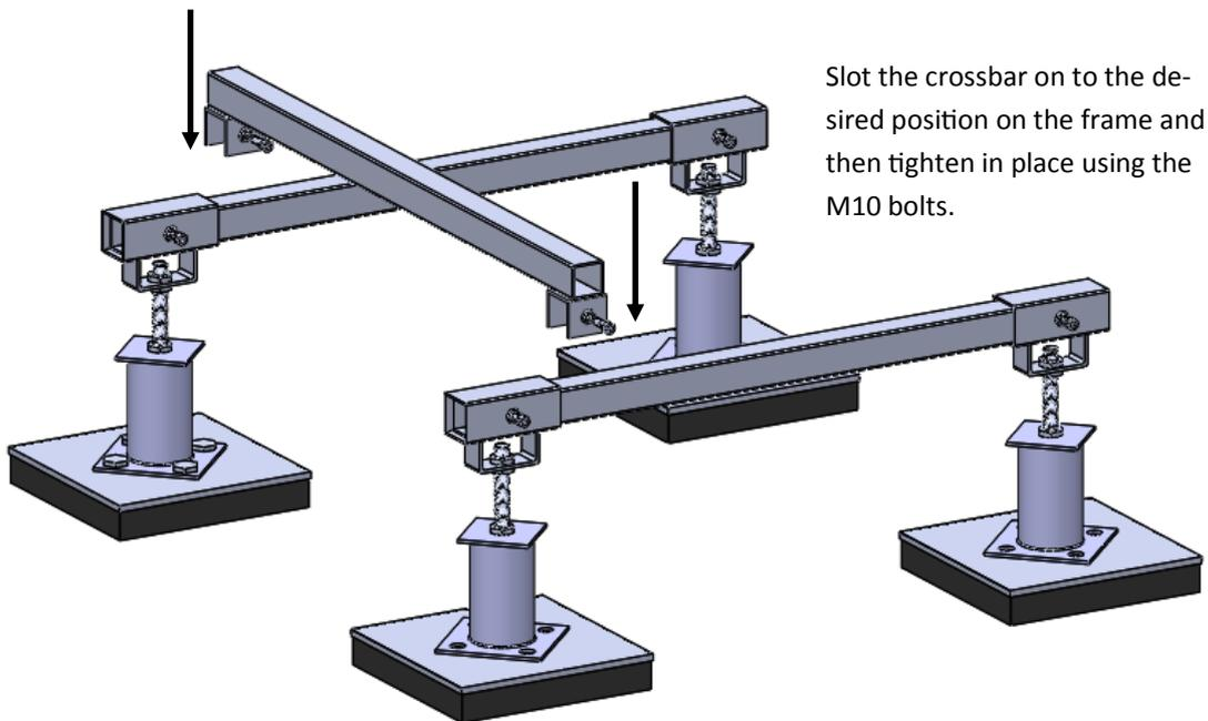
Slot the crossbar on to the desired position on the frame and then tighten in place using the M10 bolts.
