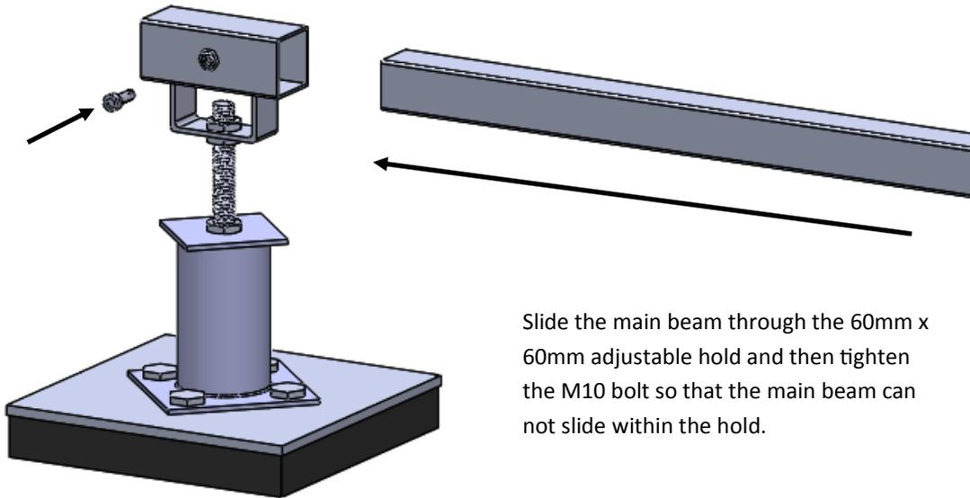
Slide the main beam through the 60mm x 60mm adjustable hold and then tighten the M10 bolt so that the main beam can not slide within the hold.
