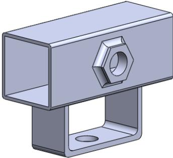
A 60mm x 60mm hold is welded onto a U beam which sits at the top of a support foot. Main beams slot through this hold and are held in place by an M10 bolt.
