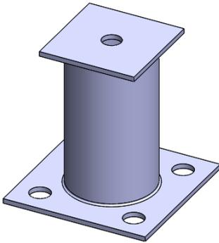
The 90mm diameter x 150mm length tube is bolted into the 300mm x 300mm galvanised steel plate and foam base using 4 M10 bolts. It also holds the threaded rod through the top central hole using two nuts.
