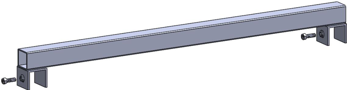
A cross bar consisting of a coupler (the amount dependant on frame configurations) and a main beam, held in position by M10 bolts as before. There is one M10 bolt per coupler.
